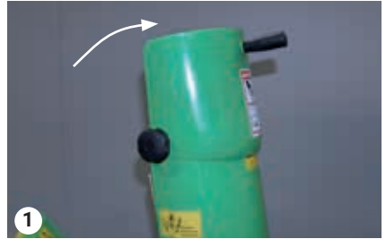
Adjust the spout so that it is completely upright
