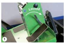
Transport lock in locked position
