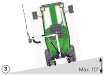
Do not drive on slopes with an incline of more than 10°
