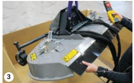
Lift out mower with crane or forklift
