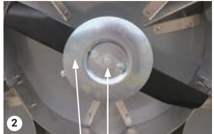
2 Plate, bolts and locking ring
