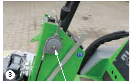
Turn the throttle until it is half open
