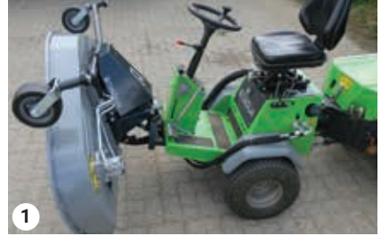
1 Flip the mower forward
