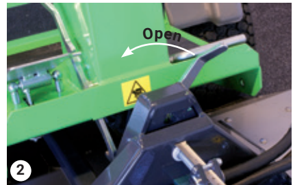
Locking handle on the A-frame – open
