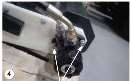
Loosen the nuts holding the oil motor in place, 2 pcs
