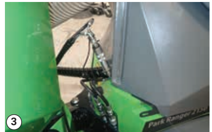
Attaching the hydraulic hoses from the hopper to C connector
