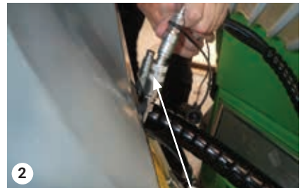
Mount the small hoses from the Weed brush on the hopper connectors
