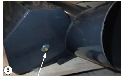
Loosen the bolt holding the centre brush in place
