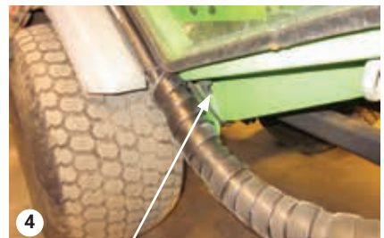
The hoses are fastened with a rubber strap
