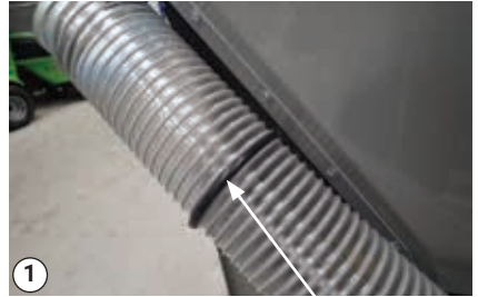
Rubber ring mounted on suction hose
