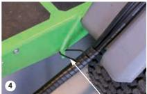
The hoses are fastened with a rubber strap
