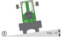
Do not drive on slopes with an incline of more than 10°
