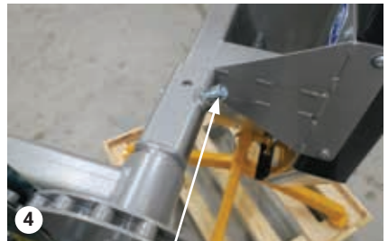
Tighten the allen bolt. Check the trimmer can not move at all from the trimmer arm square pipe.
