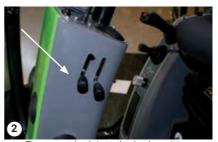
Transport lock in unlocked position
